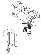
Adjust delay action accordingly to obtain desired delay time from 90 to 50.
