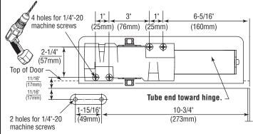
An optional mounting plate is required where the head frame face is less than 3-1/2" (89mm). Plate requires 1-3/4" (44mm) minimum head frame.
