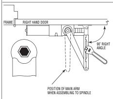
Slide connecting rod into forearm of main arm. Rotate main arm until connecting rod is at a 90° angle to frame. While holding arm in this position, tighten down forearm screw.
