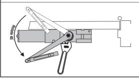
Use adjustable wrench to rotate spindle 45° counterclockwise for Right Hand Door or clockwise for Left Hand Door. Place main arm on spindle so that it is 45° or less from the tube end of the closer body. Secure main arm and spindle by tightening spindle bolt.
