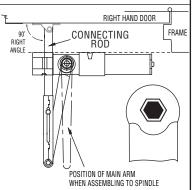
Slide connecting rod into forearm of main arm. Rotate main arm until connecting rod is at a 90° angle to frame. While holding arm in this position, tighten down forearm screw.
