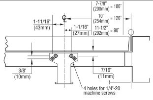
Select hand of door. Fold template on the hinge edge of door line. Fold or cut upper corner illustrated on template and align template with the hinge edge of door. At the "Frame Stop Line" fold toward you and attach template to door. Mark, prep and drill/tap 1/4"-20 holes for closer body and parallel arm bracket mounting screws.
