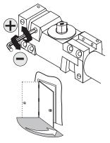
**Note:** Adjust closing time speed from 50 to 0. Greater closing times may be required for elderly or handicapped.
