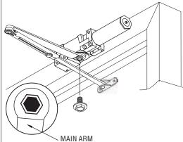
Orient main arm 90° from the closer body. Press arm down on spindle and secure with spindle bolt.
