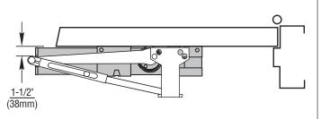
Rotate main arm until the pivot point is 1-1/2" from door surface.
