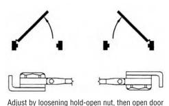
to desired position and tighten hold-open nut securely.
