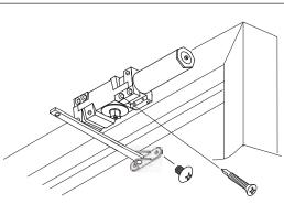
Remove template and use mounting screws to install the closer body to the top jamb and the connecting rod shoe to the door. Closer body should be oriented so that the tube end of closer is toward the hinge stile.
