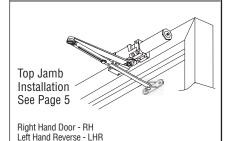
• These door closers should **NOT** be installed on the exposed side (weather side) of exterior doors.
