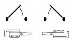
Adjust by loosening hold-open nut, then open door to desired position and tighten hold-open nut securely.
