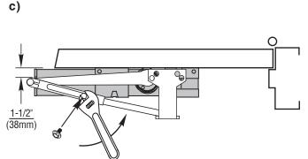
While holding arm in this position, tighten down forearm screw.
